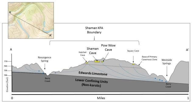
Figure 25. Geologic cross section of the Shaman Cave KFA.
