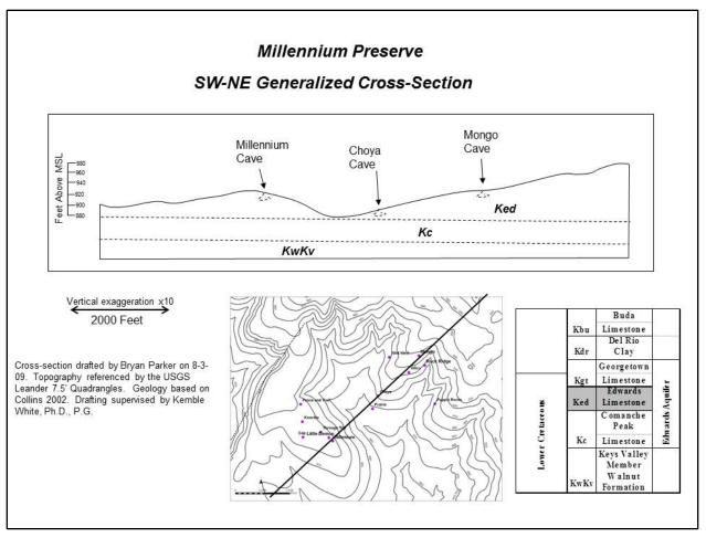
Figure 11. Millennium Preserve showing geological cross section.
