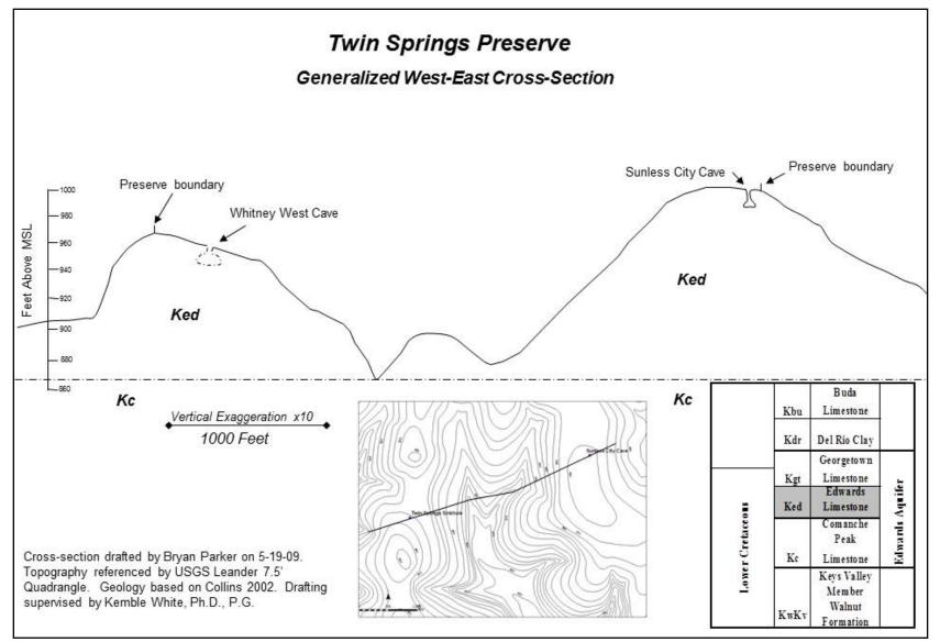
Figure 3. Twin Springs KFA geologic cross section.
