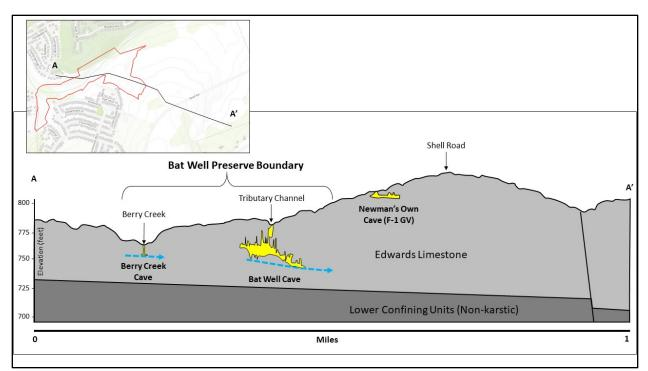
Figure 27. Geologic cross section of the Bat Well Cave Preserve.
