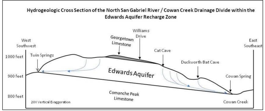
Figure 18. Cat and Duckworth Bat Caves hydrogeologic setting with local springs.
